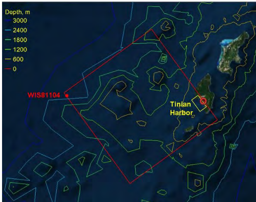
Figure A19. Wave model grid boundaries at Tinian Harbor.
