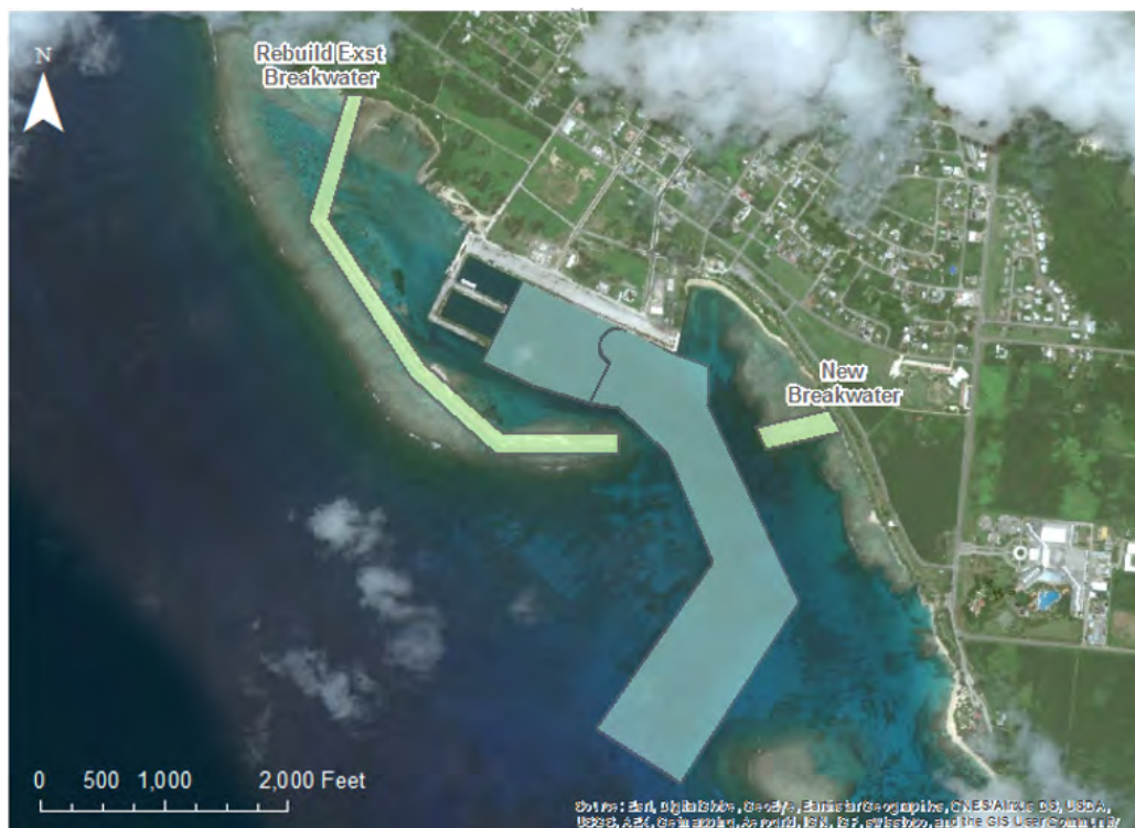
Figure A16. Conceptual Layout of Rebuild Existing Breakwater and Add New Breakwater.
