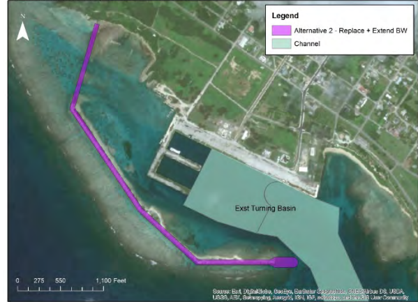
Figure ES-2. Replace and Extend Existing Breakwater in Place
