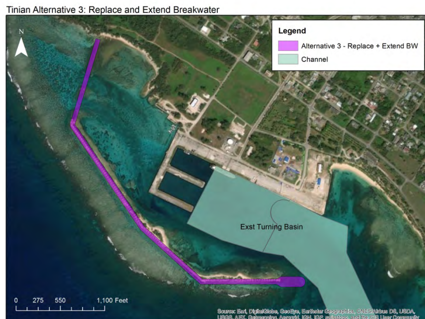
Figure 4-2 Conceptual Layout of Alternative 3 – Replace and Extend Existing Breakwater along Current Alignment
