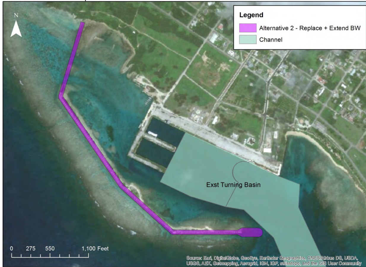
Tinian Alternative 2: Replace and Extend Breakwater
