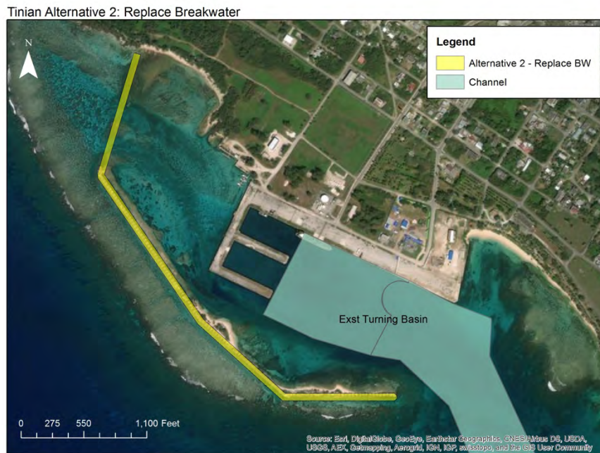
Figure 4-1 Conceptual Layout of Alternative 2- Replace Existing Breakwater along Current Alignment
